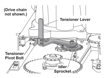
Loosen the tensioner adjustment bolt jam nut and advance the adjustment bolt until it contacts the tensioner pivot bolt nut. This will keep the pivot bolt from moving.
