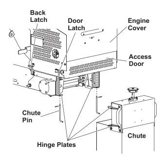
3. Line up the hinge pivot holes. Insert a 1/2" x 8-1/4" chute pin on each side. Secure the chute pins with 3/32" x 2-1/4" cotter pins.
