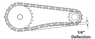
To increase engine chain tension: Loosen the four bolts that secure the engine mount to the engine base and pull the engine away from the clutch. After correct tension is achieved, retighten the engine mount bolts.
