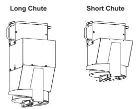
Ideal spinner height is 12"–18" above the ground. For some installations the chute length may need to be adjusted to achieve the desired spinner height.
