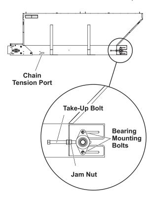
4. Tighten the bearing mounting bolts.
