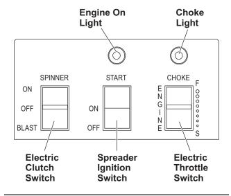
NOTE: The conveyor and spinner will operate when spinner switch is in the "ON" or "BLAST" position.
