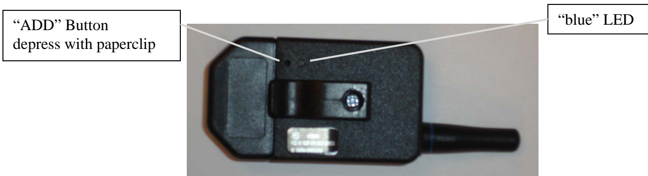
Fig. 1: Keyfob Back Button Assignments
