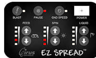
Pause LED On, Spreading stopped
