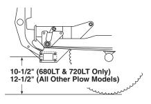
The recommended push beam height for the 680LT & 720LT undercarriage assembly is 10-1/2" from the center of the push beam to level ground.
