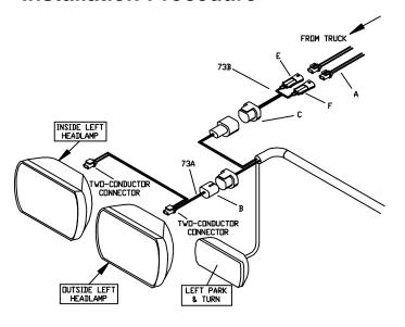
Figure 1. '04 & Newer Titan Headlight Adapter Connections G10161
