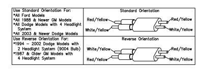
Figure 3. Vehicle Option Connector
