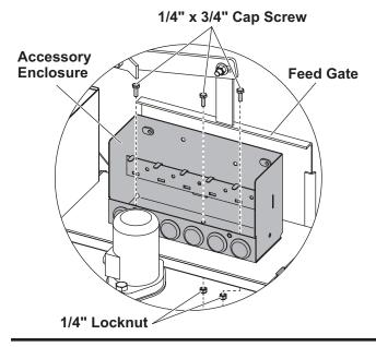
One of the two supplied fuse holders will serve as an isolated stud block. Install the isolated stud block to the accessory enclosure as shown using two #10 x 1/2" machine screws and #10 locknuts.
