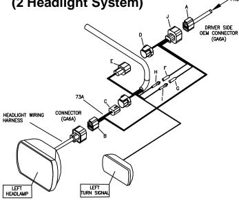
Figure 1. Driver Side Single Connections
