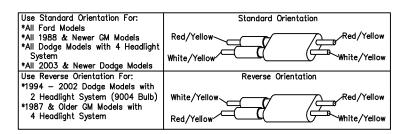
Figure 3. Vehicle Option Connector
