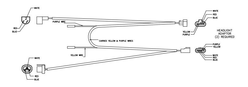
Figure 1. Headlight Adapter Kit, 2003 & Newer GM C4500/C5500
