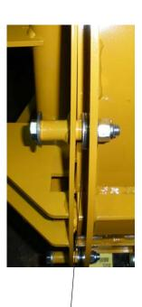
Wing Pivot should be shimmed with 1/2" washers supplied to keep the pivot parallel with the moldboard.
