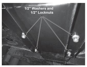
10. Fasten the skid plate assembly to the bracket assemblies installed in Steps 3 and 4 using one 1/2" x 1-1/4" cap screw and 1/2" locknut per side.
