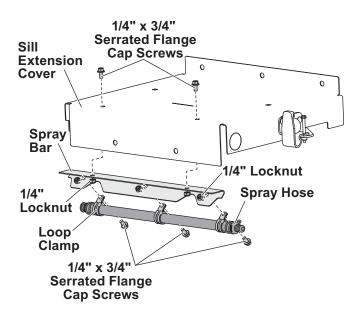
4. Connect the spray bar hose to the hose that exits through the rear face of the pump box. Position the spring clamps at each end of the hose.
