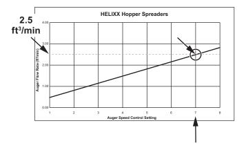
On the Optimal Flow Rate table on page 17, find the Delivery Flow Rate value (previously determined in Step 2 (2.5 ft³/min) and the Application Rate (8 gal/ton). 4. Find the point at which these two values meet on the table (see example below). This box shows the Optimal Flow Rate for this liquid application (0.74 gal/min).
