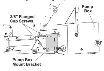
4. From the passenger's side of the spreader, find the two 3/8" flanged cap screws that fasten the extension cover to the auger. Remove the 3/8" flanged cap screw that is closest to the hopper body.
