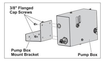
5. Slide the pump box mount bracket assembly onto the two 1/2" bolts, replace washers and lock washers and tighten the nuts.
