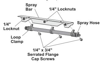
3. Use two 1/4" x 3/4" serrated flange cap screws with 1/4" locknuts to fasten the spray bar assembly to the sill extension cover as shown.
