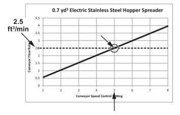
On the Optimal Flow Rate table on page 17, find the Delivery Flow Rate value (previously determined in Step 2 (2.5 ft<sup>3</sup>/min) and the Application Rate (8 gal/ton). 4. Find the point at which these two values meet on the table (see example below). This box shows the Optimal Flow Rate for this liquid application (0.74 gal/min).
