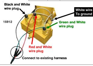
Note: Do not use couplers (22443 and 22444) on units installed on E-Z Mount Plus, MDII or Drive Pro Plow Systems. Use 1/4 x 33" Hose Assy SAE 6 x Face Seal. (eliminates coupler use on both the ange cylinder hoses and P.A. Block)
