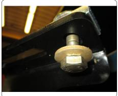
Secure all M12 fasteners with socket wrench. A 19mm end wrench may be used to secure forward most bolt.
