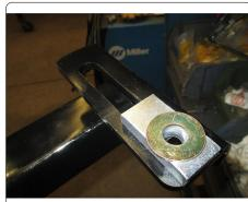
4. Insert one (1) M12 hex bolt with one (1) 1/2" conical toothed washer through side plate, CM-SP52 spacer and 1/2" flat washer into each rear most weldnut.
