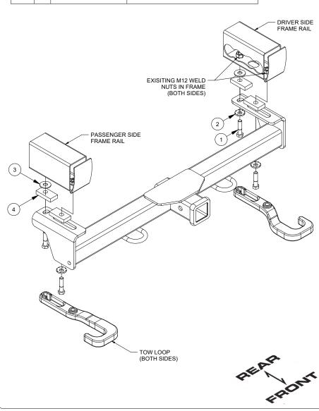
1. Remove two (2) hex bolts and one (1) tow loop from bottom of each frame rail and return to vehicle owner. These will be replaced with the included M12 hardware.
