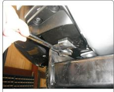
6. Torque all M12 fasteners to 86 ft-lbs. Use a 19mm socket torque adapter to torque front bolts.
