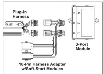
For vehicles with headlamp bulb or turn signal daytime running lights (DRLs): The DRL wire from the plug-in harness will not be used. Coil and cable tie the DRL wire.
