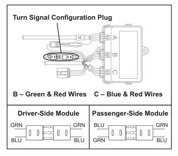
2. Connect the single-wire connector from the vehicle lighting harness to the single-wire connector from the plug-in harness.
