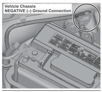
NOTE: Do NOT route the black vehicle battery cable wire to the NEGATIVE (-) battery post. See the note on page 12 for more information.
