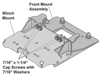
Secure the winch mount attachment arms to the front mount assembly by installing four 3/8" x 1-1/4" cap screws (two per side) through the attachment arms of the winch mount. Secure each cap screw with a 3/8" locknut. Hand tighten.
