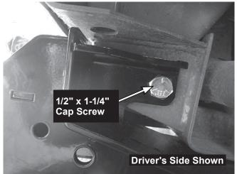
Install a 1/2" x 1-1/4" cap screw with a 1/2" washer through the rear hole of the mount on the driver's side. Secure with a 1/2" washer and 1/2" locknut. Hand tighten.
