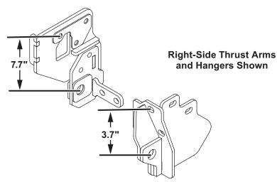
77596 (shown) Thrust Arm, Right 77595 (not shown) Thrust Arm, Left 77598 (shown) Hanger, Right 77597 (not shown) Hanger, Left
