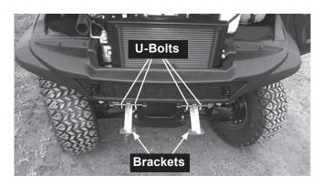
7. Fasten the passenger-side and driver-side radiator brackets (if installed in Step 4) to the top of the brackets installed in Step 6, using a 3/8" x 1-1/4" cap screw with a 3/8" flat washer on each one. Secure each cap screw with a second 3/8" flat washer and a 3/8" locknut. Tighten the fasteners hand tight.
