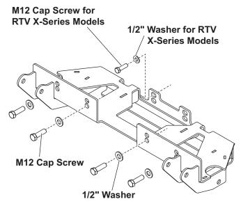
18. Tighten all fasteners according to the torque chart.
