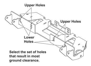
4. Install the rear edge of the mount to the skid plate using the supplied M10 cap screws and 3/8" washers. Insert the fasteners through the set of holes in the mount that align with the holes in the skid plate.
