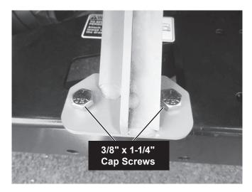
Place a bolt bar through the cap screws on the inside of the brush guard and secure with two 3/8" locknuts. Tighten hand tight.
