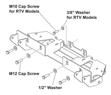
5. Tighten all fasteners according to the torque chart.
