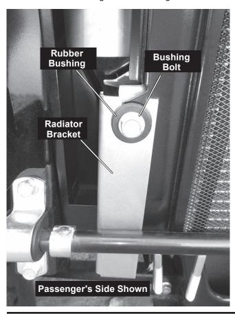
Starting on the passenger's side of the vehicle, install two U-bolts over the cross member found below the radiator. Position the U-bolts on either side of the frame member that runs fore and aft, as shown below.
