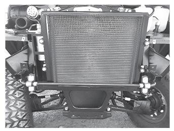
2. Remove the two carriage bolts that secure the top of the radiator frame. Remove the two carriage bolts that secure the bottom of the radiator frame.
