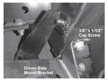
4. Install a 3/8" washer and 3/8" locknut on the cap screw and hand tighten.
