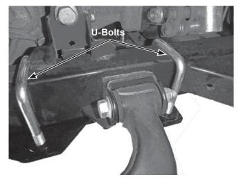
10. Secure each U-bolt with two 3/8" locknuts. Tighten according to the torque chart.
