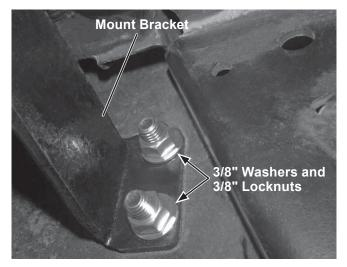
7. Clamp the rear of the skid plate assembly to the vehicle frame. Adjust as necessary so that the skid plate is centered. Tighten all fasteners installed above according to the torque chart.
